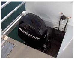
Electric tilt toggle is located on the left side of the engine, below the cowling (cover).
